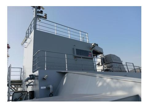
3. **Bridge control stations**: there are 3 on the BRF navigation bridge, enabling the crew to check refuelling distances (port and starboard stations) and RAM configuration (main station).
